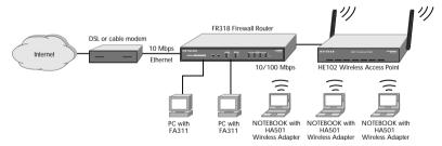
If you are running a wireless network in infrastructure mode, please set up the access point (such as the NETGEAR HE102 802.11a Wireless Access Point) first, before you set up this wireless adapter.
